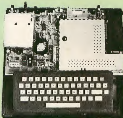
Photo 3. Inside the computer, left to right: transformer and AC power supply under an insulating shield; +5, -5 and +12 regulated power supplies (including heat sinks); cassette and joystick circuitry (at back); RF modulator (metal box at back); interference shield (large metal cover); and cartridge slot.
